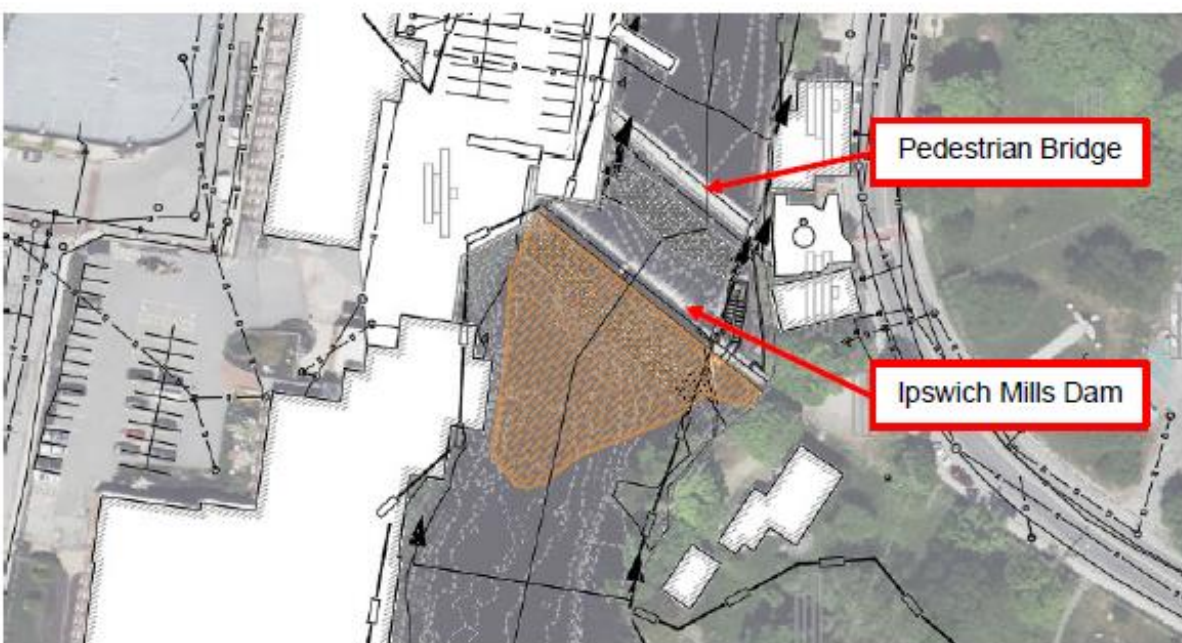
Figure 23. Approximate Extents of Anticipated Coarse Sediment Transport Immediately Upstream of Ipswich Mills Dam
